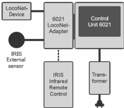
**Note:** One or more devices such as keyboards, memory or switchboard can be attached between the Control-Unit and the Adapter as long as the Adapter is the last unit in the chain.
