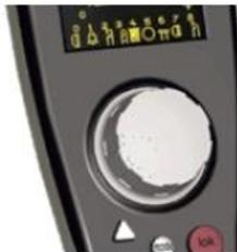
Rotating the throttle serves to change the speed of the locomotive. Pressing on the throttle serves as emergency stop of the actual locomotive and, when in AC – throttle mode (Factory setting), to change the direction.
