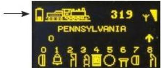
Radio reception (only DAISY II Radio) shows the quality of the radio reception (Signal strength). If "?-ERR" appears during operation in place of the address the radio reception is interrupted.
