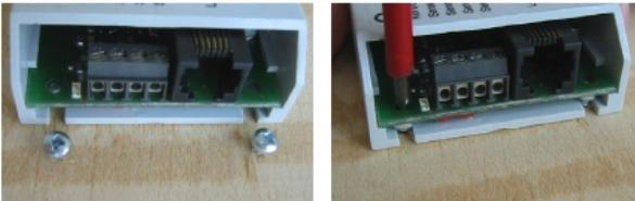
Mount the MARCo receivers under the layout in proximity to the track sections. For this you position the MARCo-Receiver under the layout baseboard. Mark the mounting hole of the module. Turn two round screws (round head  $\varnothing 2.5 \times 10$ ) far into the board so that the notches in the MARCo-Receiver slide over the screws. Then turn the screws tight.
