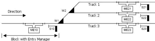
At the entrance into the station there is a single approach track with the signal S10. The approach track is a block section with a MARCo-Receiver set up as the automatic *Entry manager*. This regulates the entry of the train to the designated track.
