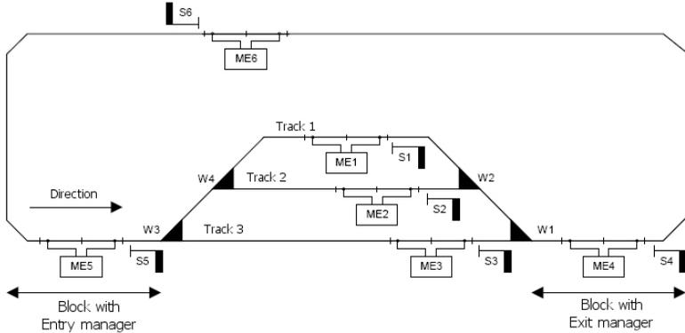
The connecting track has yet another MARCo-Receiver LE6 to manage that block section. This results in three block sections between the stations entry and exit. The automation is done by means of the following programming:
