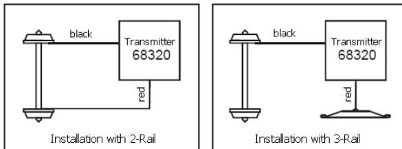
Connect the wires from the MARCo transmitter with the power pickups of the locomotive: The red wire to the right (insulated) of pickup and the black to the left (non-insulated) pickup.
