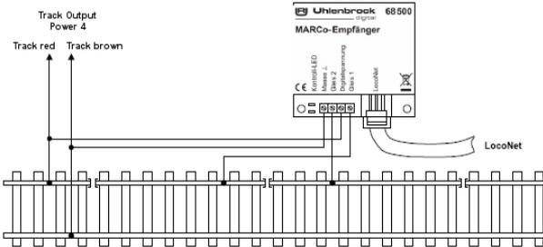
The feedback message for the track section should be via feedback address 10. The MARCo-Receiver has module address 2 and works as a block section with block status reporting. Its exit signal has address 1.
