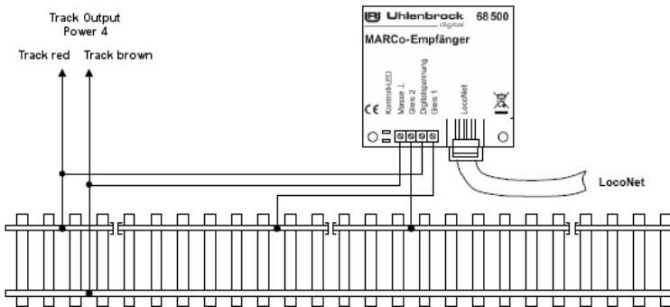
**Note:** If multiple boosters are used then take care to ensure that the chassis connections of all the transformers are connected together, to ensure trouble free operation.
