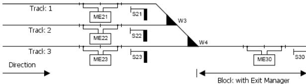
Different trains are located in the station waiting for the exit signals to turn green, which can happen manually. They monitor the state of the section, i.e. the block section following the station. If this block is vacant, i.e. no vehicle is in the block, a train from the station can depart and enter this block. To do this, switch all appropriate turnouts to the exit and lastly the exit signal of the desired station track, to green.
