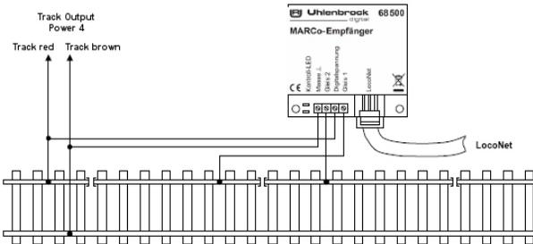
The feedback for the track section uses an address over 50. Furthermore upon entry to the section, route 3 from group 2 in the Intellibox is to be enabled, if a train from category 3 enters the section. Locomotive 100 is to set the exit signal for the track with the solenoid address 30 to "green".
