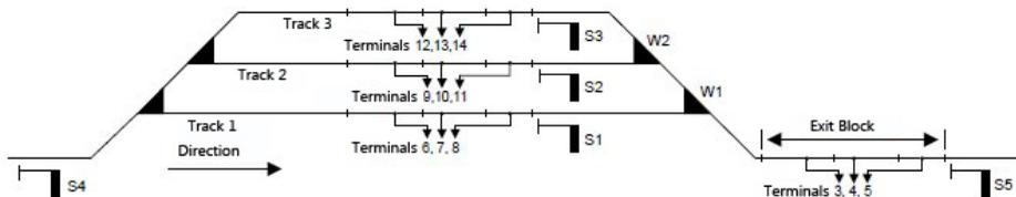
By programming individual LocoNet CVs (LNCVs) the following settings can be made in the station control with automatic exit.
