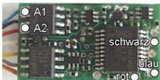
Additional special functions such as smoke generator, telex coupling or driver compartment lighting can be connected to the special function outputs A1 and A2. The feed to the device is soldered directly to the decoder circuit board. The return line is connected either to the blue wire of the decoder or the locomotive chassis.
