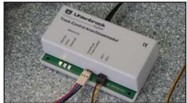
Connect the module to separate 16V AC transformer and connect the provided LocoNet cable to the LocoNet T socket of the Intellibox.
