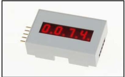
**Note:** The train number display functions only in connection with the LISSY system.
