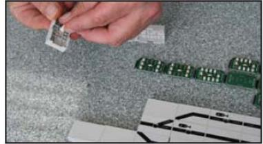
Insert the PCBs into the plastic segments where needed.
