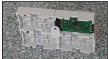
Now you can add the next plastic segments. if necessary add the connector plug for each block of four. Continue, until you have the desk assembled completely.
