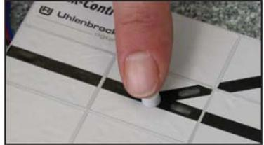
Press the key as often as required to illuminate the desired symbol for the segment to be programmed.
