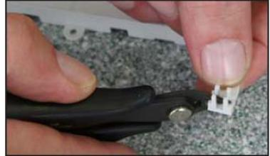
Now you can cut off all connector pins that protrude outwards with a side cutter.
