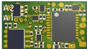
Additional special functions such as smoke generator, telex coupling or driver compartment lighting can be connected to the special function outputs A1 and A2. The feed to the device is soldered directly to the decoder circuit board. The return line is connected either to the blue wire of the decoder or the locomotive chassis.
