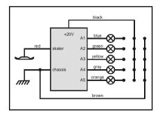
In case the attached device has a high current consumption, we recommend to fasten the decoder directly to a metal chassis frame or heat sink with hot glue. All common brands are suitable for this.
