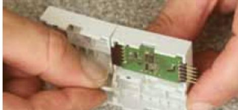
4. **Plug the** segments together and fix them in place with the enclosed connector plug. Connecting PCBs with or without indicators connects turnout or signal PCBs within a segment row. Cross jointers connect the individual segment rows to each other.
