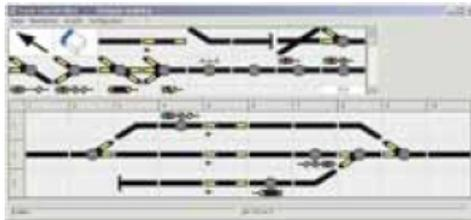
1. **Plan your** control panel with the provided planning software on the PC. Print the track plan, the connecting plan and the parts list.
