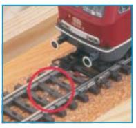
If the automatic actions are not to be dependent on the driving direction, then the two infrared sensors can be used independently on two tracks. They report the address and train class.
