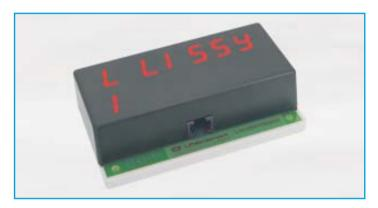
This module features a two-row LED display which can be easily read at a distance. There are 6 different display modes. One can define up to 16 different custom displays by setting up specific parameters for each display mode. Each of these custom displays can easily be selected by using turnout commands.
