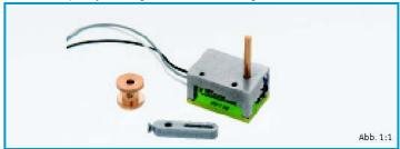
To motorize vehicles and working models, e.g. crane cars, pantograph raising, gantry cranes or gate motors. The motor has torque of 0.12 Ncm and can lift a weight of 60g with the pulley. Load free speed of 30 rpm.
